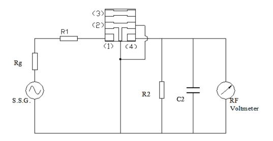
R1=280Ω (1±5%,) R2= 330Ω (1±5%,) Rg=50Ω; C2=10pF (Including stray capacitance and input capacitance of RF voltmeter), S.S.G: Output Voltmeter; (1): Input; (2): Ground; (3): Float; (4): Output
