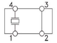
Pin 2 and Pin 3 are not connected to the GND
