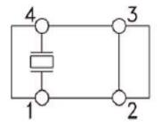
Pin 2 and Pin 3 are not connected to the GND
