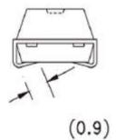
Note: Metal (Crystal inside) may be exposed on the top or bottom of plastic case. That will not be affect performance and reliability of the part in use.
