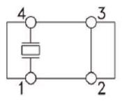
Pin 2 and Pin 3 are not connected to the GND
