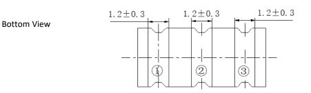
Connection: (1) Input (2) Ground (3) Output
