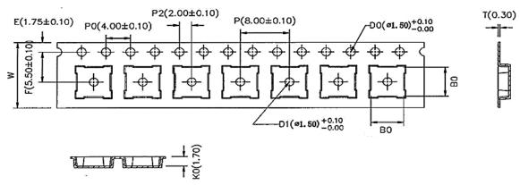
\* B0: 5.35 for QCC8C; 4.15 for DCC6/QCC8B; 3.35 for DCC6C/QCC8D
