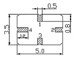
PIN NO.CONFIGURATION1Input/Output3Output/Input2, 4Case Ground
