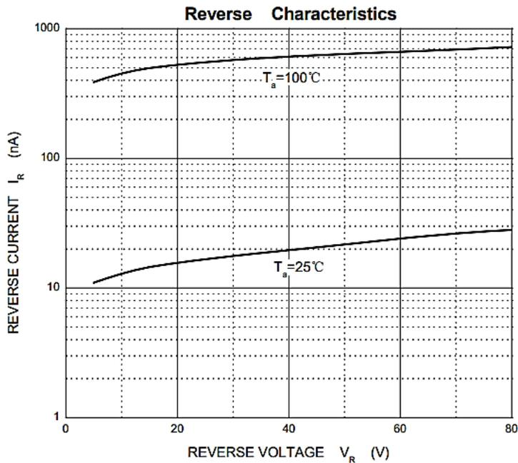
**RATINGS AND CHARACTERISTICS CURVES-** For Reference Only,  $T_a=25^\circ\text{C}$  Unless Otherwise Specified.
