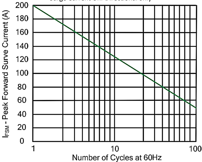
Figure 8 - Maximum Non-Repetitive Forward Surge Current Uni-Directional only
