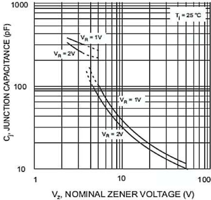
Fig. 5 Junction Capacitance vs Nominal Zener Voltage
