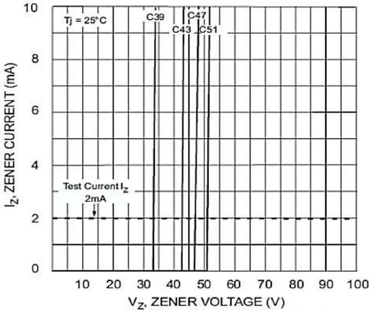
Fig. 4 Zener Breakdown Characteristics
